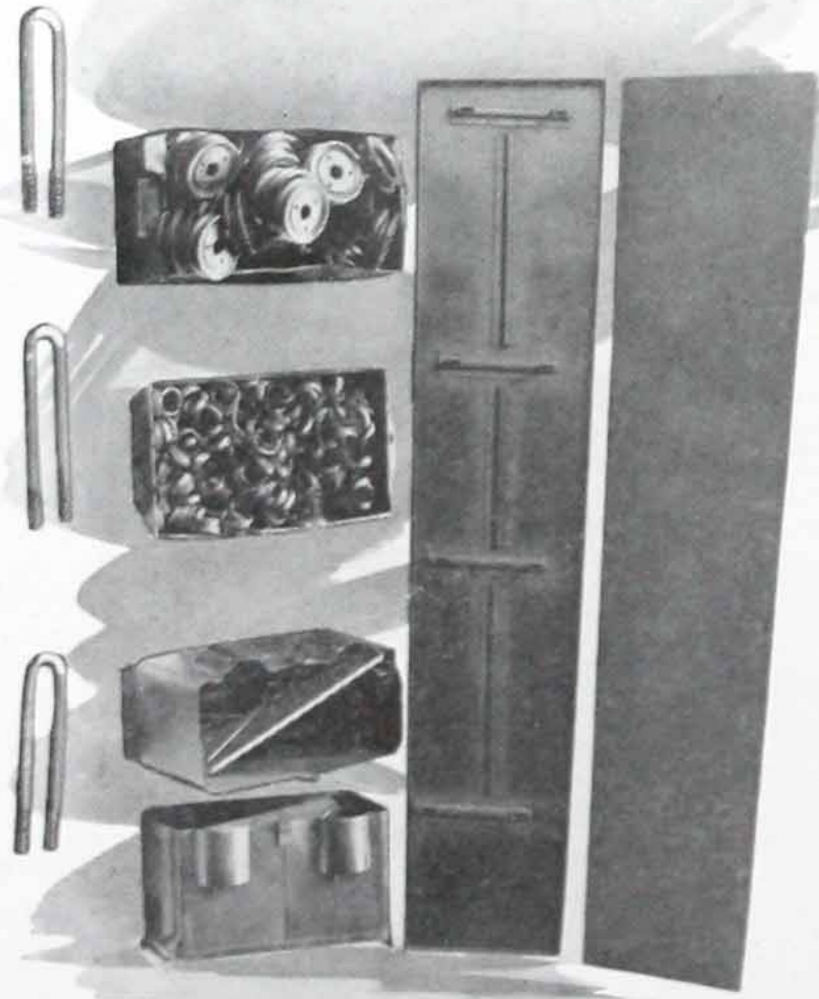
Parts Rustproofed by the Parker Process
